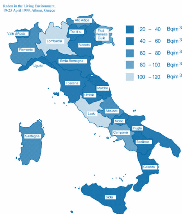
Figure 1: Map of average annual radon concentration in all the 21 Italian Regions as estimated from the National Survey. The actual regional average values of Trentino Province, Alto Adige Province, and Sardegna are significantly higher than the mapped values (see text).
